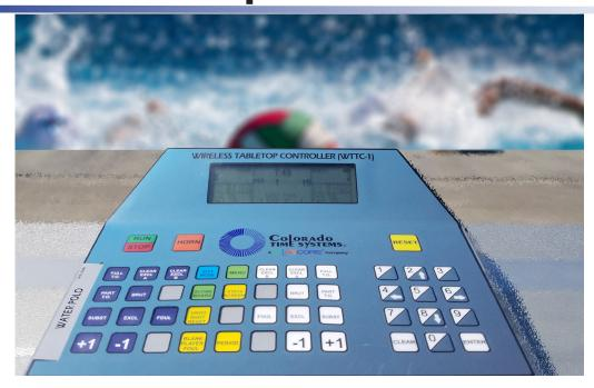
The wireless tabletop controller features an operating distance up to 1,000 ft., buttons with tactile dome feedback, and a large transflective LCD screen that is easily readable in all environments from darkness to bright sunlight. The controller includes a built-in real time clock to keep time of day.
